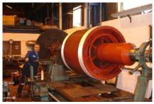
We have fully equipped Machine shop facilities available for all types of machining, milling, welding, radial drilling, metal spraying & balancing. This section also has one of the largest centre lathes available within the industry allowing machining of large armatures, shafts and rotors.
